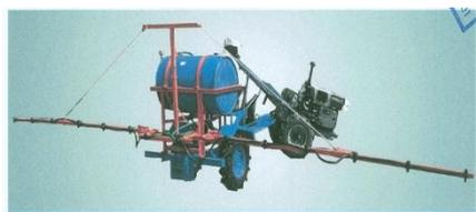
(57) The invention relates to a sprayer attachment for tractors, featuring foldable sprayer arms for versatile use, easy storage and transportation. The attachment includes a mounting frame, fluid reservoir, pump system, and a folding mechanism that allows the sprayer arms to retract towards the center. This design enhances the ease of use, storage efficiency, and versatility of the equipment, making it ideal for agricultural spraying tasks.
